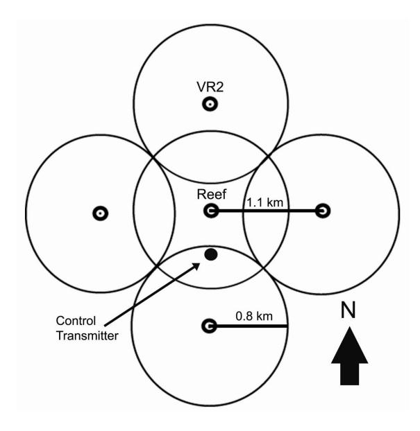
Figure 2. Receiver array design for each site, with one receiver at the reef and four others surrounding the reef 1.1 km (0.4 km at site A4) away to the N, S, E, and W. Circles represent detection range of 0.8 km. A stationary control transmitter was placed 400 m S of reef (150 m at A4).
