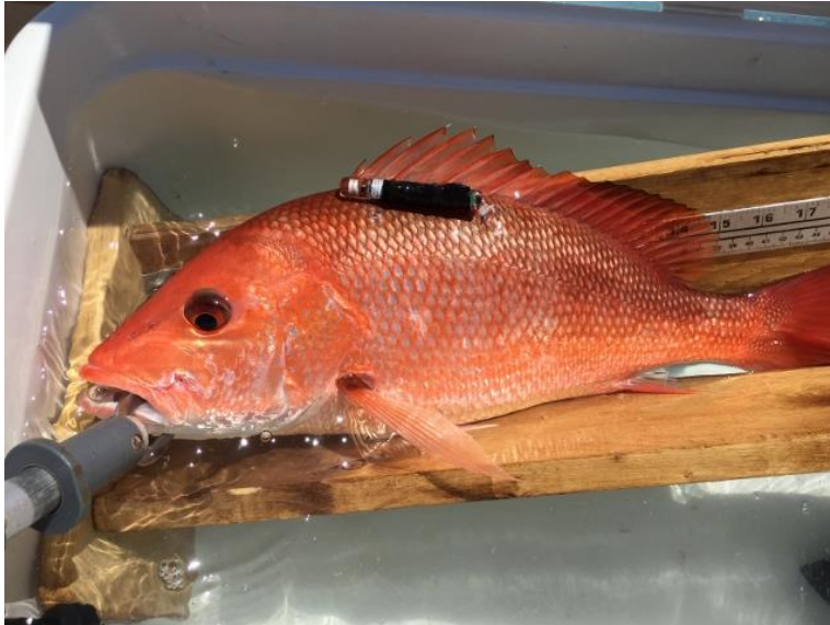
Figure 3. Red Snapper positioned in tagging/measuring cradle with Lotek ultrasonic acoustic transmitter (MM-MR-11-45-PM) using external tagging procedures
