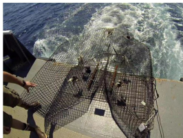
Chevron trap with mounted cameras, baited with clupeoids. (photo credit SCDNR MARMAP)
