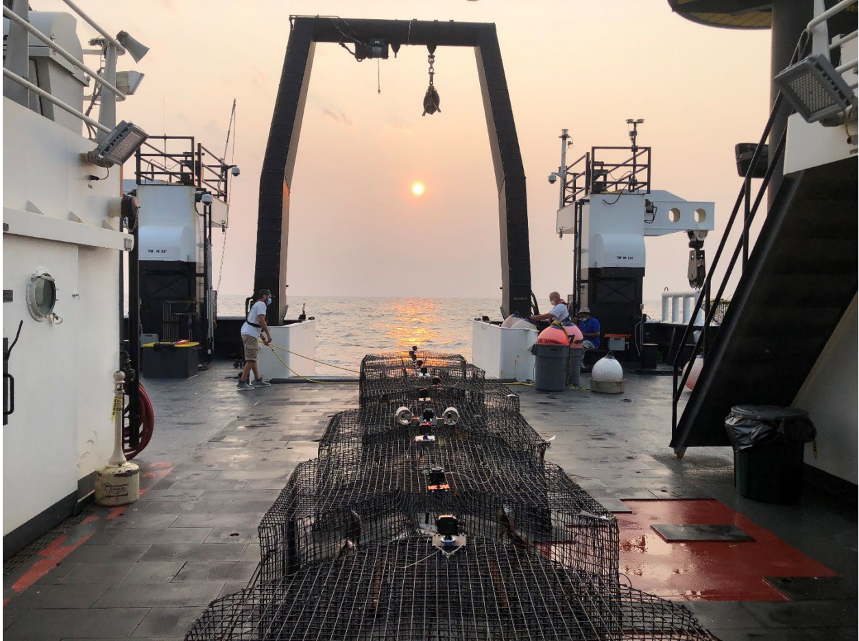
Figure 1. Chevron traps used by SERFS showing the GoPro cameras over the trap mouth and nose.
