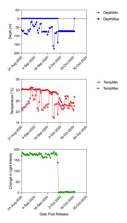
C\_lim03\_P: PSATLIFE tag recovered with 28 days of archived data reveal consistent changes in depth, temperature, and light level, indicating **survival**.
