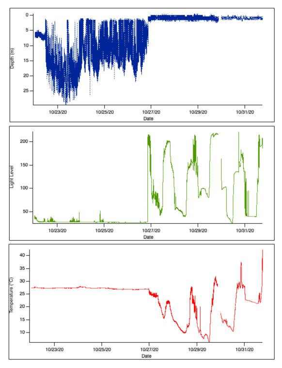
**S\_mok01\_P con't:** Transmitted data for sPAT tag showing high resolution depth data, daily changes in light intensity, and daily min and maximum temperatures and depth values for the full deployment. The constant depth (mortality) can be seen at far left of top graph.
