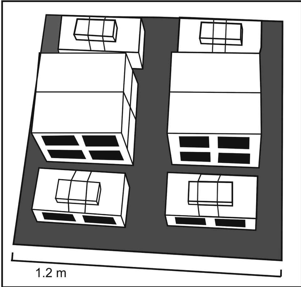
Figure 2. Artificial reef design indicating the placement of 12 concrete blocks on the plywood base and four small “break-away” bricks.
