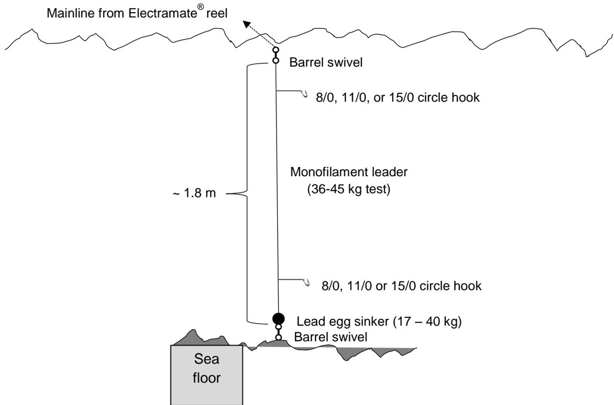
Figure 3. Diagram of terminal tackle, double-hook “chicken rig”, used during FWC RTD hooked-gear surveys along the Atlantic coast of Florida (2018).
