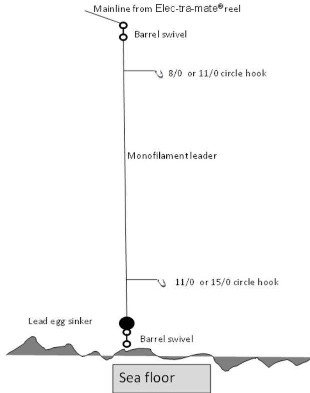
Figure 8. Diagram of terminal tackle, double-hook “chicken rig” used during FWC fisheries-independent hooked-gear (RTD) surveys along the Atlantic coast of Florida (2016).
