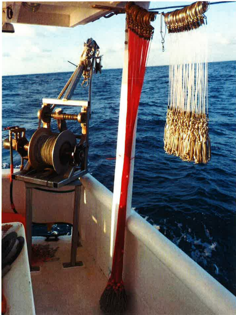
Figure 3: Comparison of Gear A (right) and Gear B (left – red monofilament leader).
