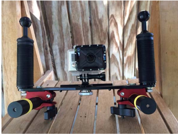
Figure 4.14.3. Materials used for rigging the video camera and underwater lasers for calibration of images
