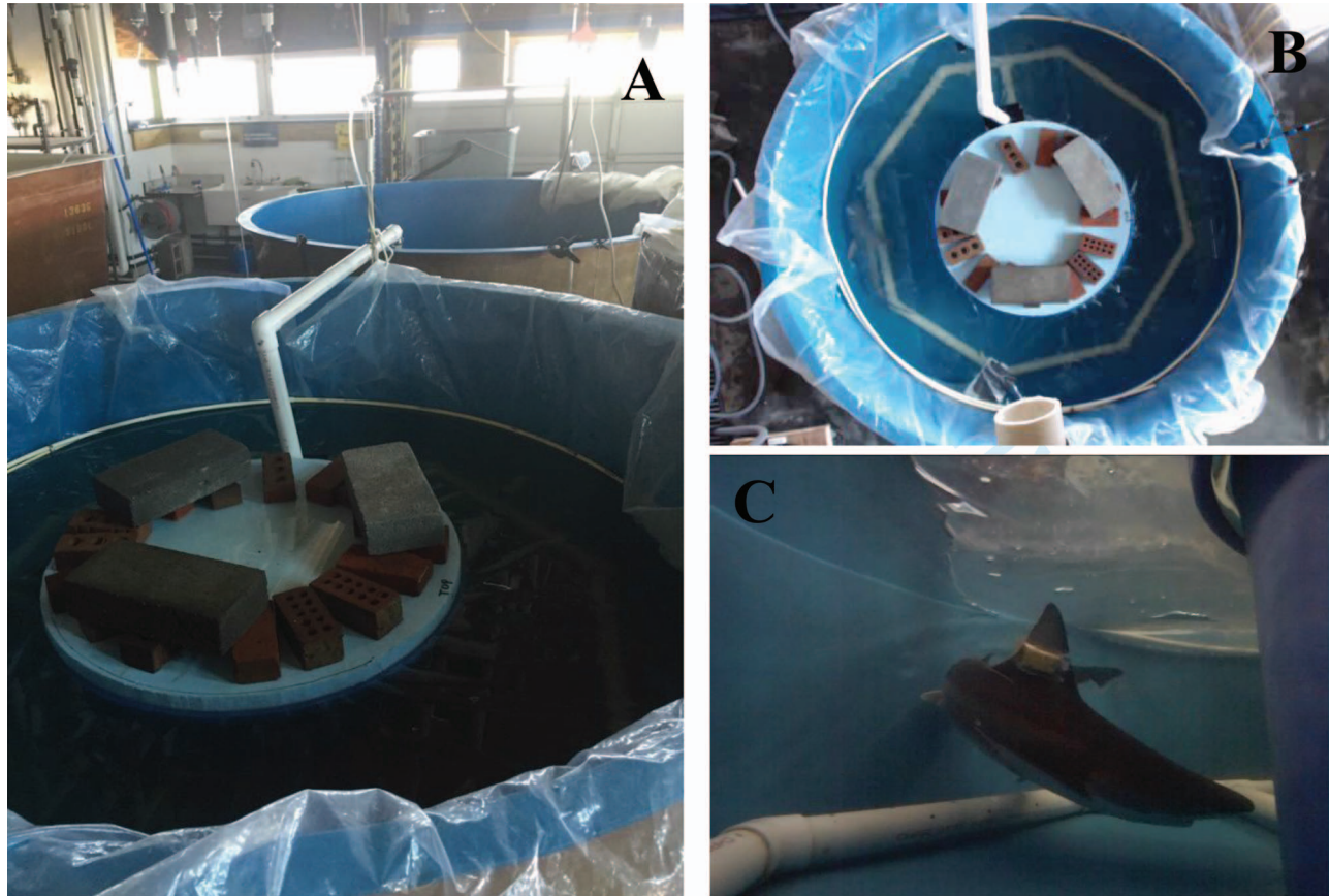
Figure 1: (A) The sandbar shark respirometer system with the respirometer in the foreground and the reservoir in the background. A PVC pipe connects the flush pump to the diffuser in the bottom of the respirometer. (B) An overhead view of the respirometer with a shark present. The PVC octagon is the diffuser that ensures mixing during the flush cycle. (C) A shark in the respirometer with an accelerometer fitted to its dorsal fin.
