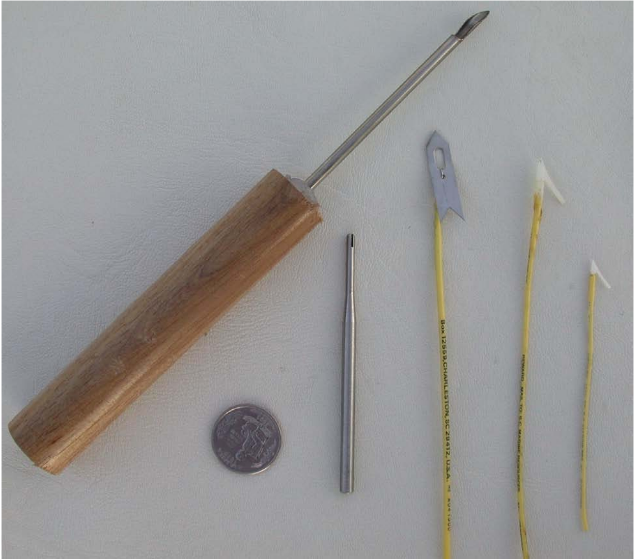
Tagging equipment, from left to right, tag applicator, stainless slotted applicator tip for use with harpoon tags, K series nylon dart tag, E series nylon dart tag.
