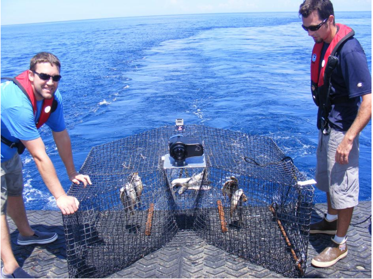
Figure 1: Chevron trap used by SERFS showing the Canon camera over the mouth and GoPro on the trap nose.
