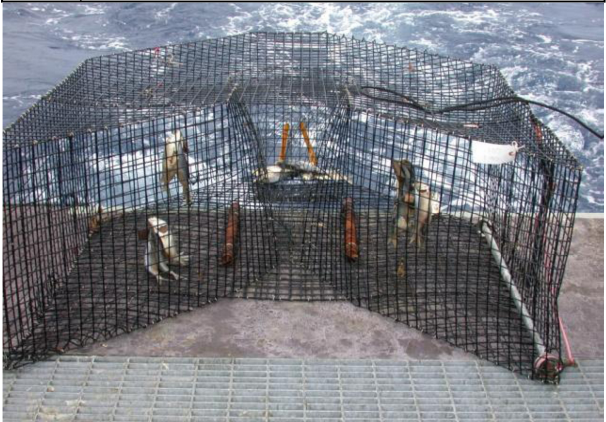
Figure 5: Chevron traps used by SERFS for monitoring reef fish. A. Diagram with dimensions. B. Chevron trap ready for deployment baited with clupeids. Iron sashes attached to the bottom weigh the trap down and help maintain the proper orientation of the trap on the bottom.
