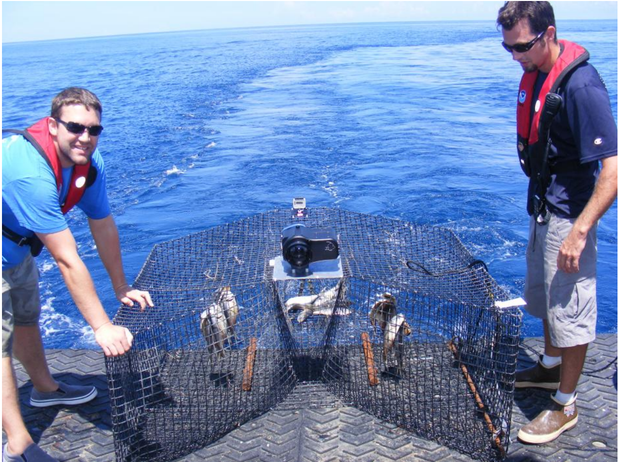
Figure 1: Chevron trap used by SERFS showing the attached underwater video cameras.
