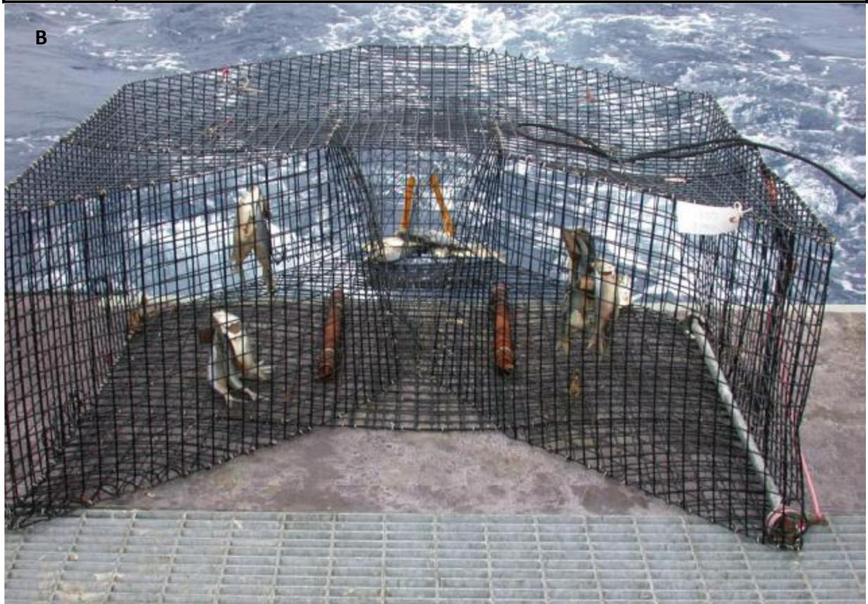
**Figure 2.** Chevron traps used by SERFS for monitoring reef fish. A. Diagram with dimensions. B. Chevron trap ready for deployment baited with clupeids. Iron shackles attached to the bottom weigh the trap down and help maintain the proper orientation of the trap on the bottom.
