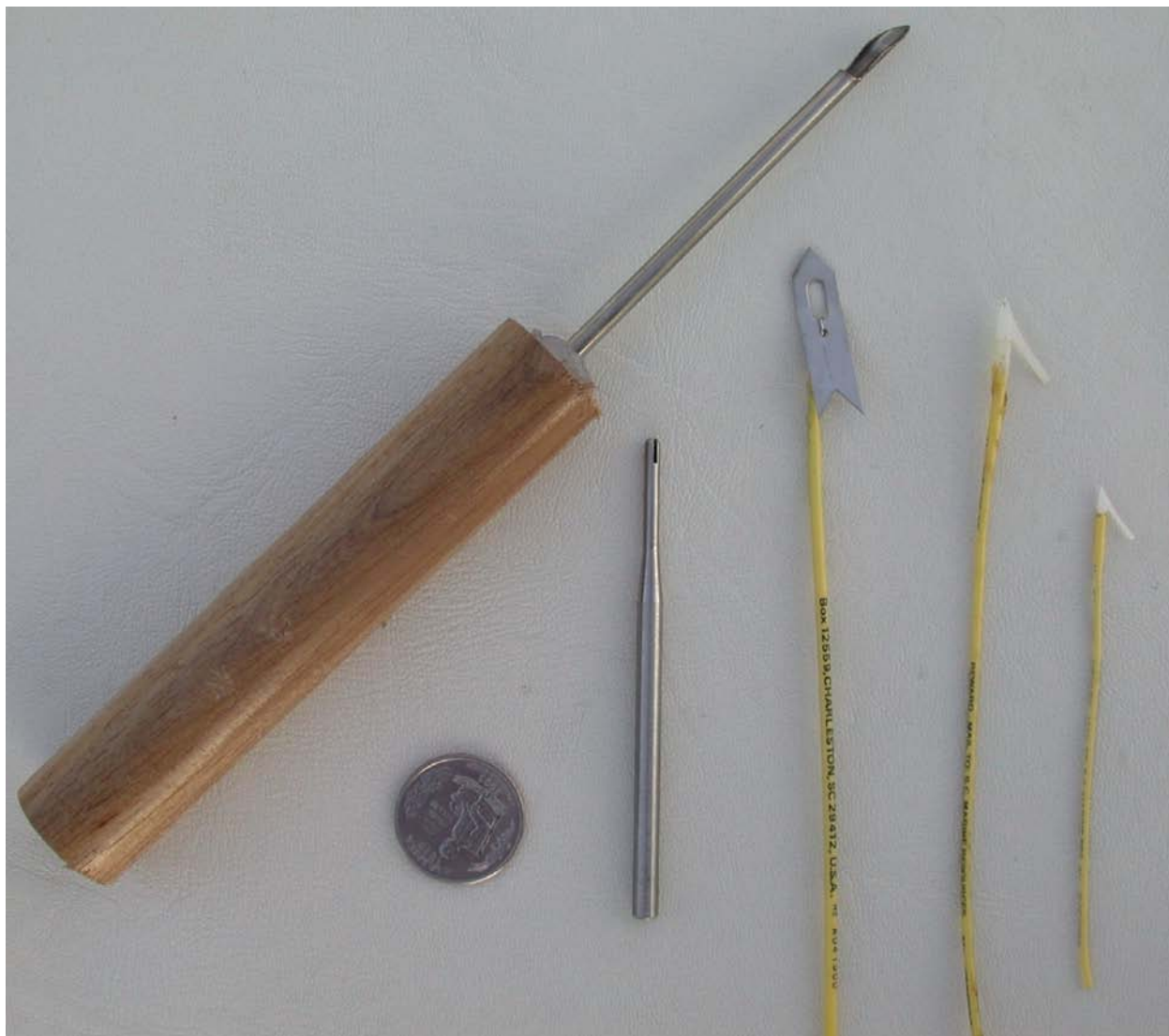
Tagging equipment, from left to right, tag applicator, stainless slotted applicator tip for use with harpoon tags, K series nylon dart tag, E series nylon dart tag.
