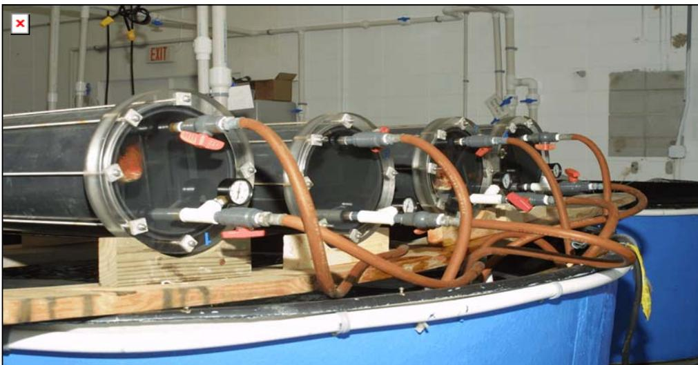
Figure 3-2. Series of fish hyperbaric pressure chambers situated over a 1,000 l tank, used in the pressure simulation experiments.
