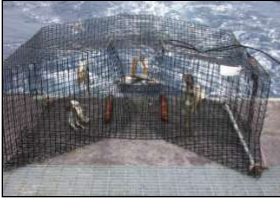
Fig. B-6. Chevron traps baited with menhaden; ready for deployment. Iron sashes weigh trap down.
