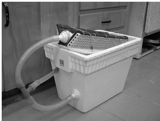
Figure 7: Photograph of the surgical platform and recirculating pump apparatus. This set-up was used to perform implantations of the ultrasonic transmitters in this study.
