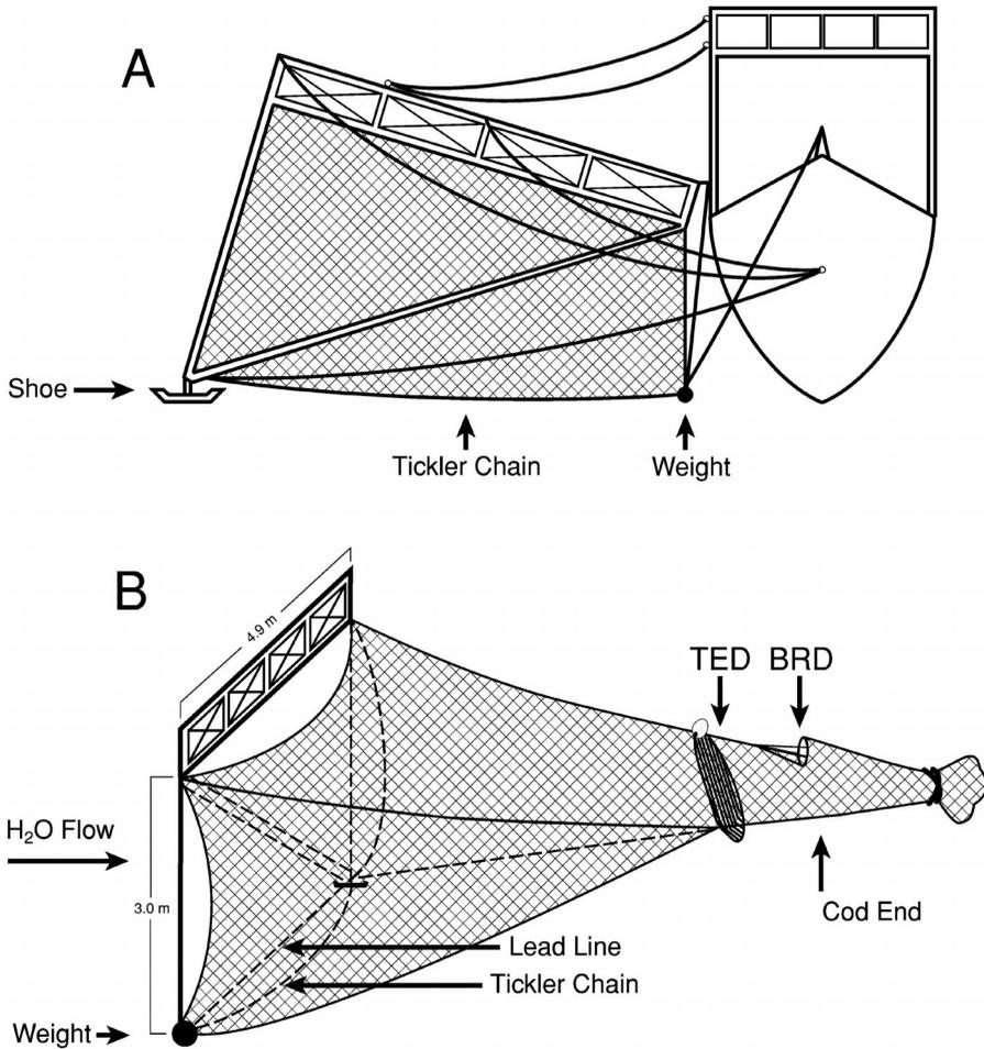
FIGURE 2.—Diagram showing (A) the skimmer trawl frame and (B) the components of the net. Both the Turtle Excluder Device (TED) and the Florida Fisheye Bycatch Reduction Device (BRD) were attached to the shrimp net.
