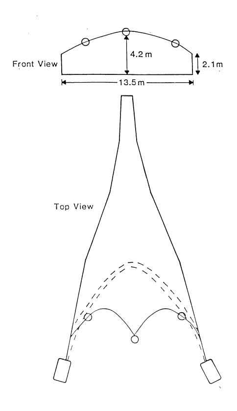
Fig. 5. Diagrammatic sketch of the two-seam trawl during tow based on results of mensuration.
