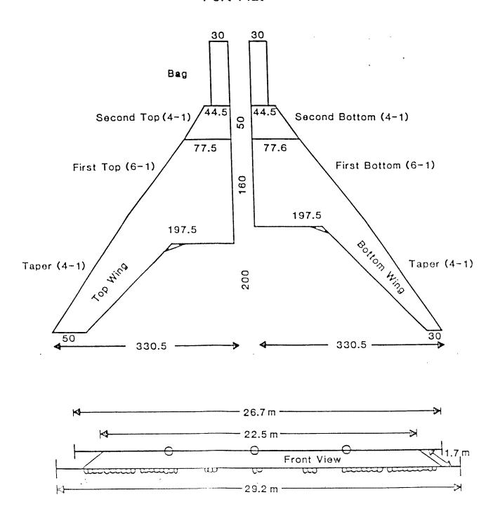
Fig. 4. Diagrammatic sketch of the tongue trawl during tow based on results of mensuration.
