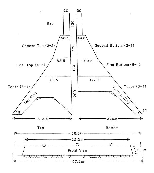
Fig. 3. Schematic representation of the two-seam trawl. Numbers with 'm' represent distances in meters, plain numbers indicate number of meshes along seam, and numbers in parentheses represent slope in meshes.
