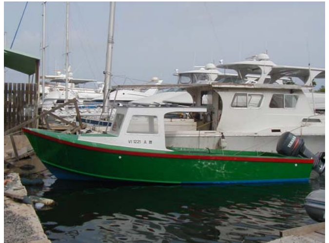
Photo 25: St. Thomas, USVI. Small single engine boat modified by the addition of a cabin.
