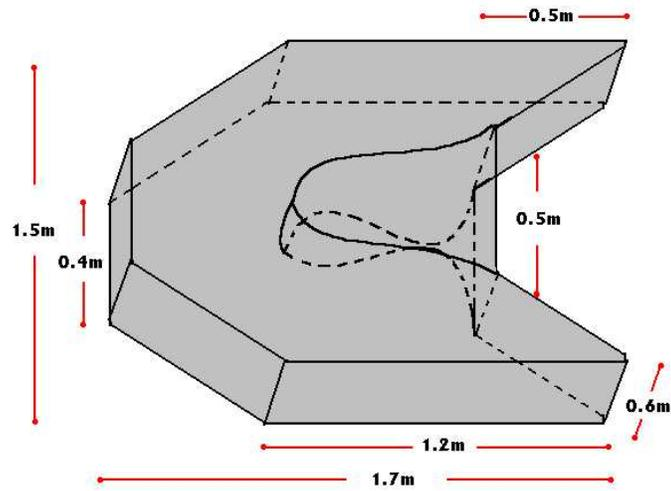
Figure 3. Detailed illustration of a chevron fish trap. The diagonal mesh size is 3.8cm.
